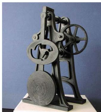
*A clock escapement mechanism: original Reuleaux model (left) and rapid-prototype model (right).*
